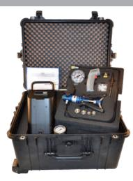
This Marine Calibration Kit enables the user to perform temperature and pressure tests, measurements and calibrations for all types of instruments. It contains a complete pressure test set as well as a temperature test including all necessary accessories and certificates according to IMO regulations.
