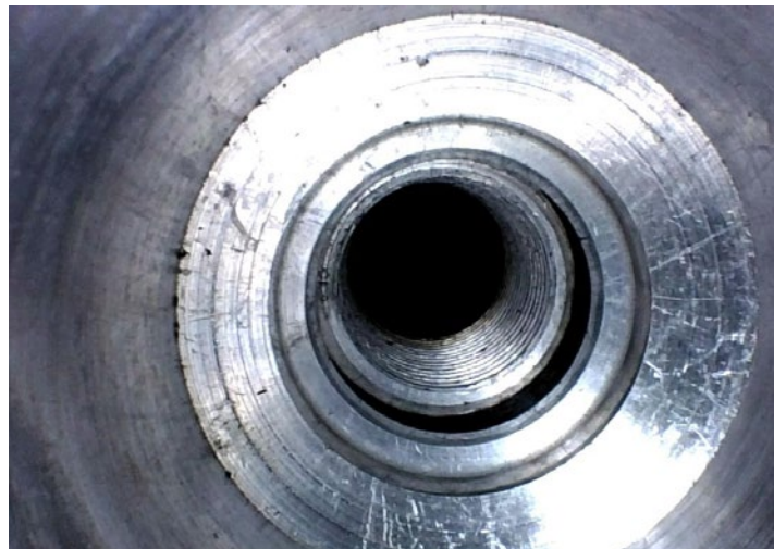
Photo above: Spark plug port inspection
